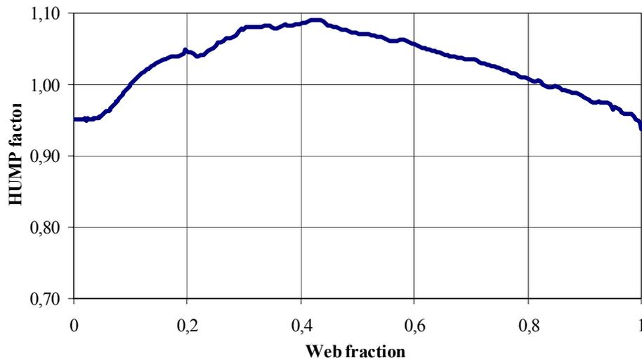
**Fig. 6.** Influence of the HUMP effect for the rocket motor *RM-2* <sup>[12]</sup>
