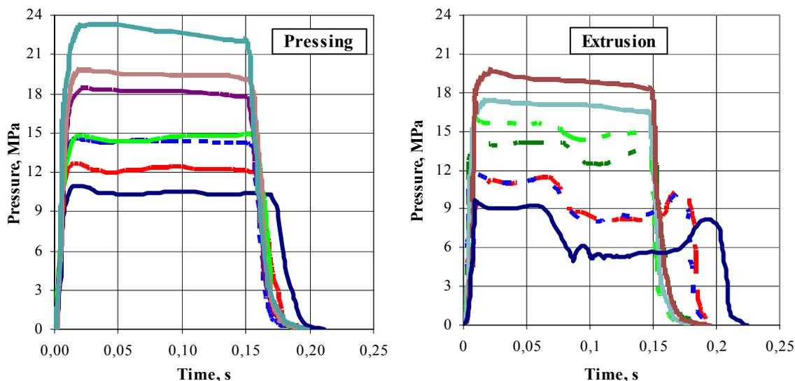
**Fig. 12.** Standardized ballistic evaluation motor 32/16 at temperature of 323 K, propellant NGR-A manufactured by pressing and manufactured by extrusion <sup>[13]</sup>
