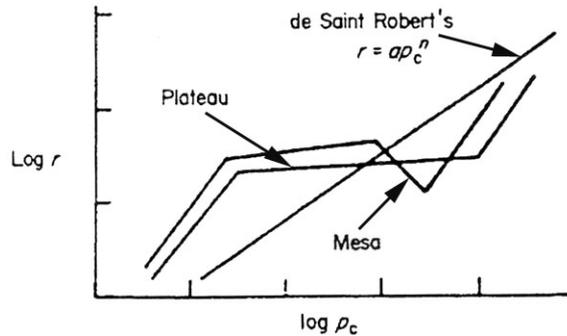
**Fig. 1.** Dependence of burning rate as a function of combustion chamber pressure<sup>[5,6]</sup>
