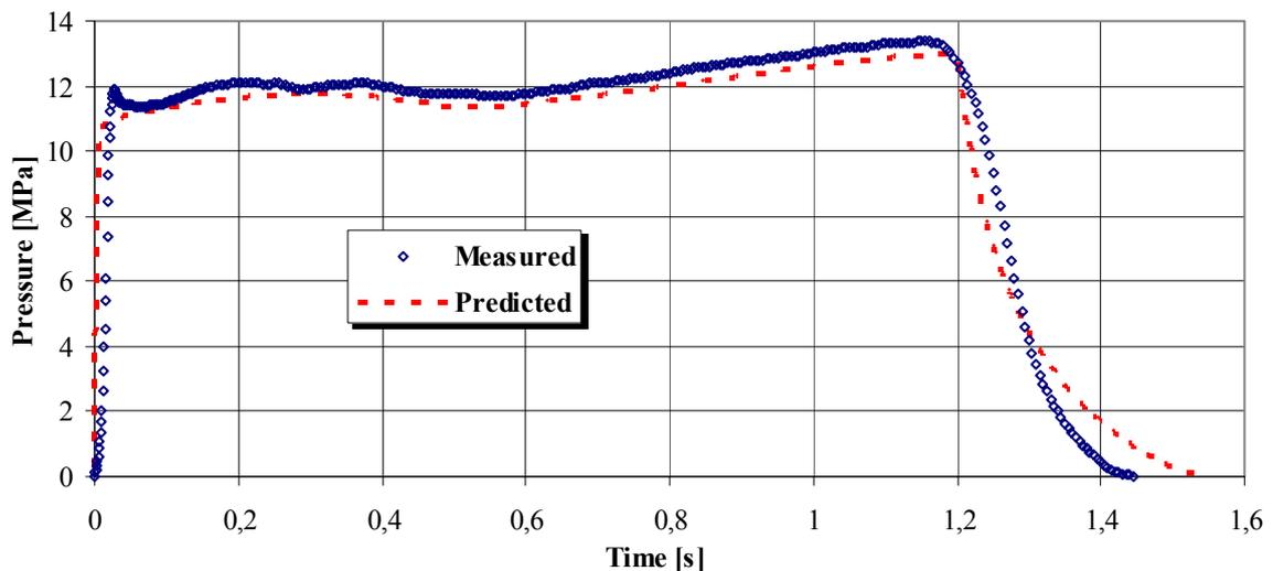
**Fig. 7.** Pressure-time curve for the motor *RM-2*, after correction due to HUMP effect <sup>[12]</sup>
