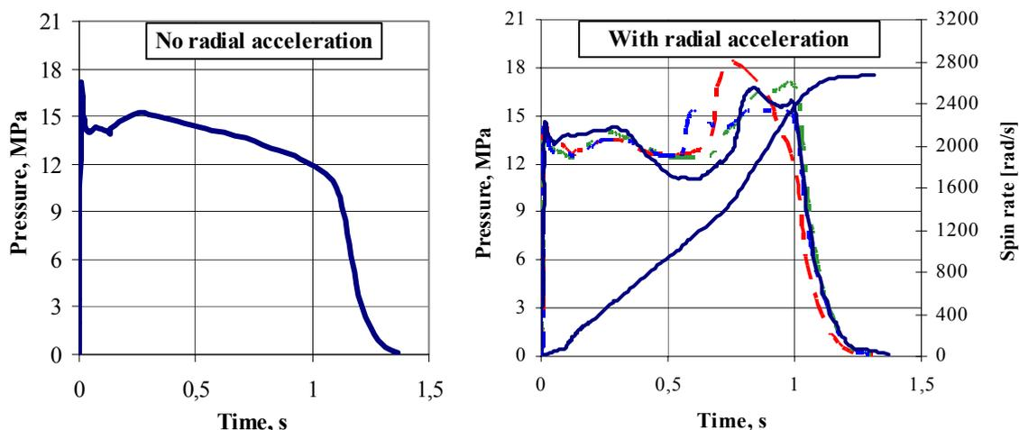
**Fig. 16.** Influence of variation of solid propellant processing on the curve pressure-time form for DB propellant NGR-A tested at temperature of 243K, without and with radial acceleration <sup>[13]</sup>
