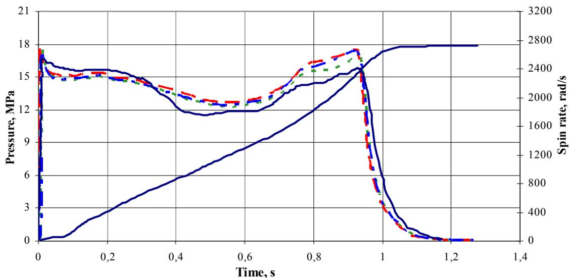
**Fig. 15.** Influence of variation of solid propellant processing on the curve pressure-time form for DB propellant NGR-A tested at temperature of 323 K <sup>[13]</sup>
