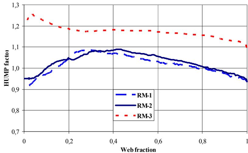
**Fig. 8.** Variation of the basic burning rate under influence of HUMP effect as a function of web thickness for rocket motors 57 mm, *RM-1* and *RM-2* (with central and multiple peripheral nozzles)
