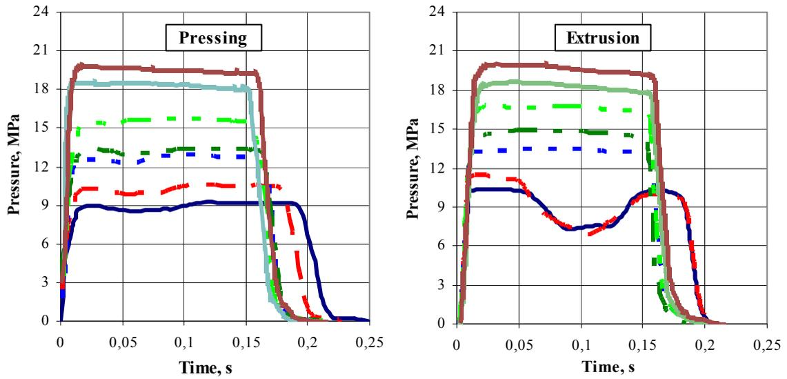
**Fig. 10.** Standardized ballistic evaluation motor 32/16 at temperature of 293 K, propellant NGR-A manufactured by pressing and manufactured by extrusion <sup>[13]</sup>
