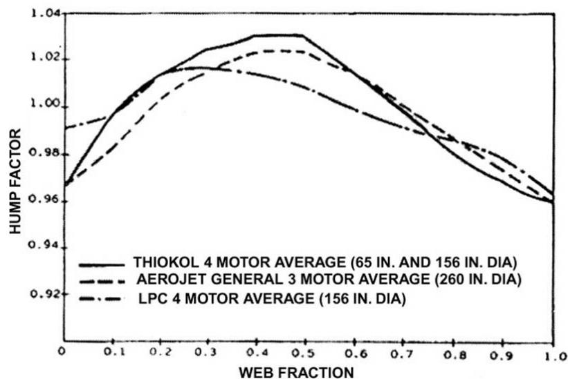
Fig. 2. HUMP factor as a function of the relative web for different rocket motors [10]
