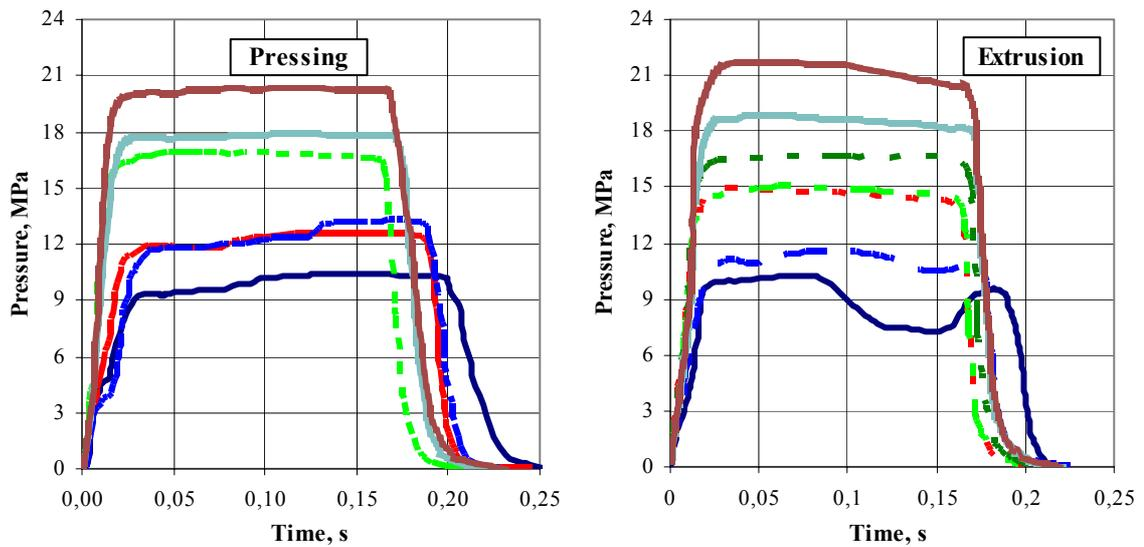
**Fig. 11.** Standardized ballistic evaluation motor 32/16 at temperature of 243 K, propellant NGR-A manufactured by pressing and manufactured by extrusion <sup>[13]</sup>
