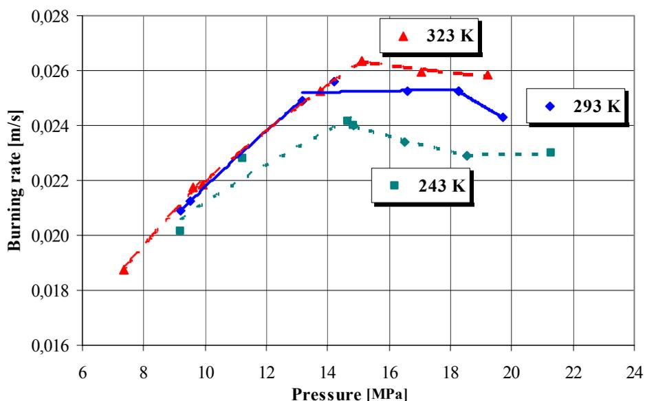
**Fig. 13.** Kinetic characteristics of the propellant NGR-A (manufactured by continuous process )
