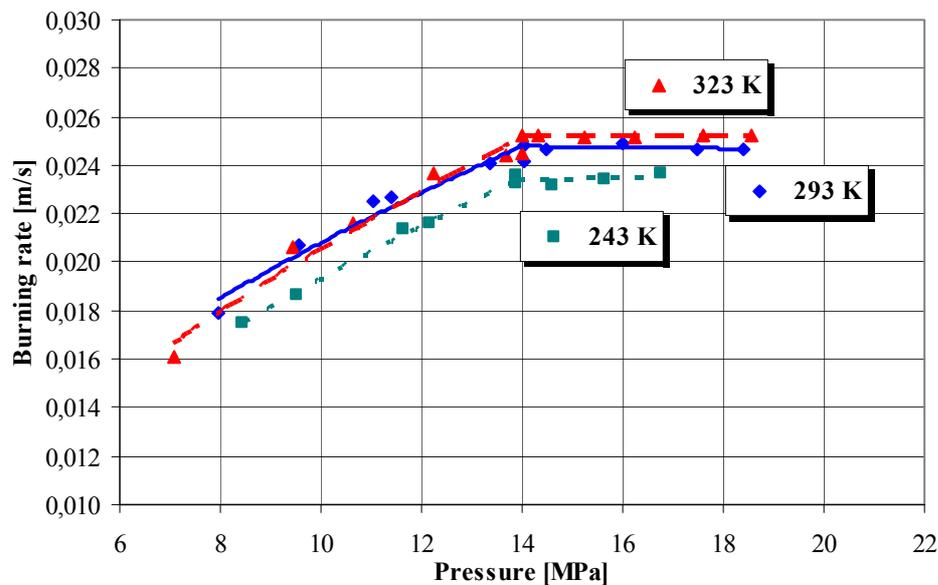
Fig. 3. Kinetic characteristics of the solid propellant NGR-A
