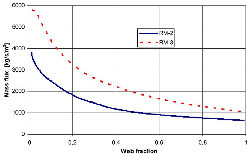
**Fig. 9.** Variation of the mass flux as a function of the web thickness for rocket motors 57 mm and *RM-2*
