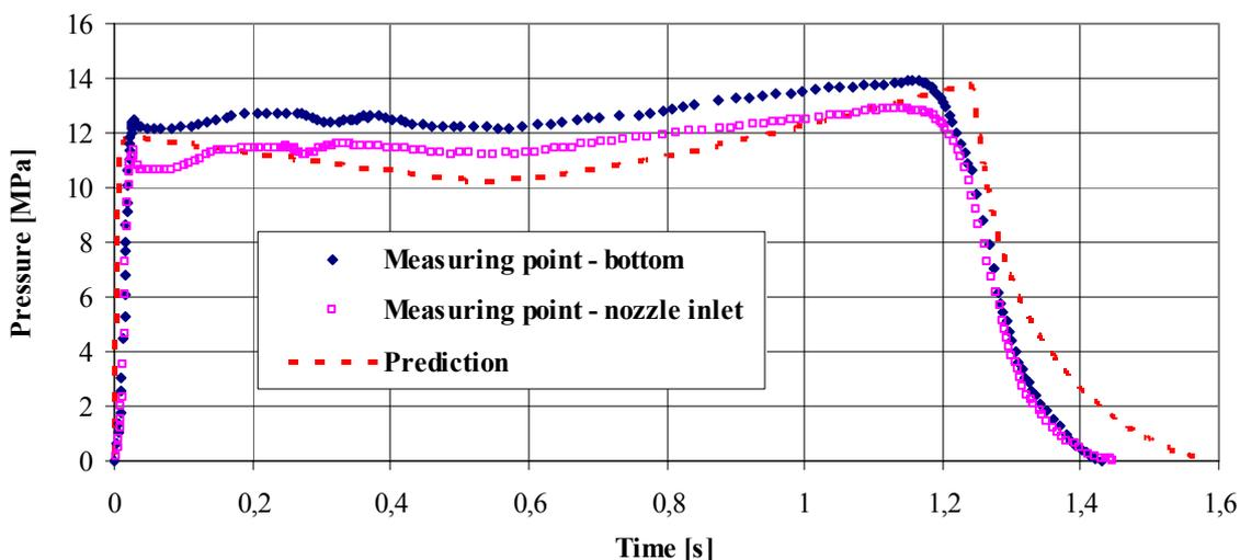
**Fig. 5.** Pressure-time curve for the test rocket motor *RM-2* <sup>[12]</sup>
