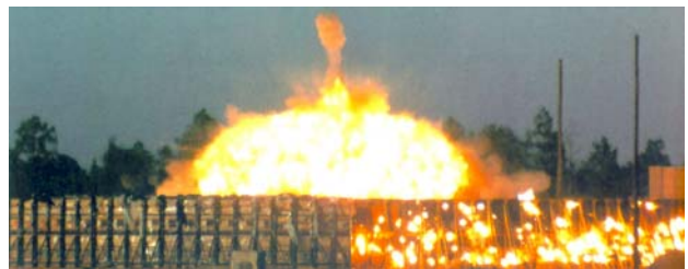
Fig. 2 Arena fragmentation test (measurement the fragments concentration density per m^2 )
