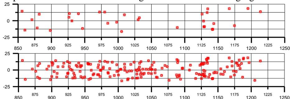
Figure 14: Dispersion of hits on horizontal target for firing times of aircraft  $t_f = 0.5$  s (fig. above) and  $t_f = 3$  s (fig. below)
