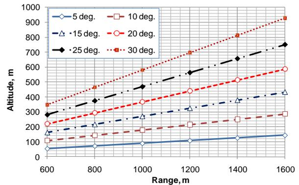
Figure 13: Change of attack height as a function of target distance and aircraft attack angle
