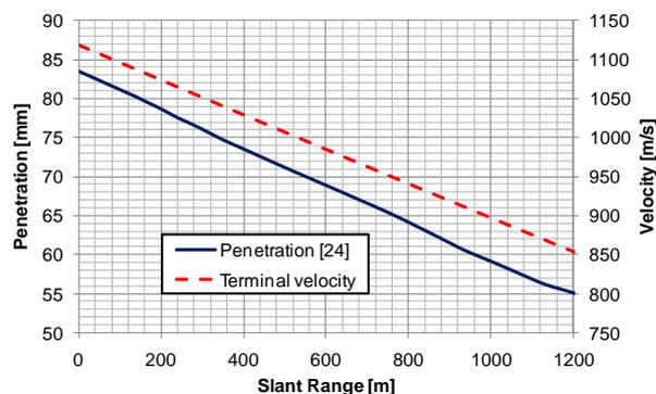
**Figure 3:** PGU-14 Penetration Results (BHN 300; 30°; 250 Kn Aircraft Launch).
