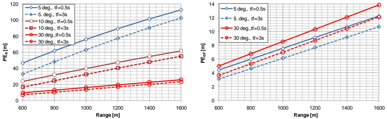
Figure 16: Probable Error for firing times  $t_f=0.5$  s and  $t_f=3$  s, in Range (left) and in Deflection (right)
