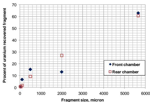
Figure 17: Aerosol vs larger fragment components of Uranium [40]
