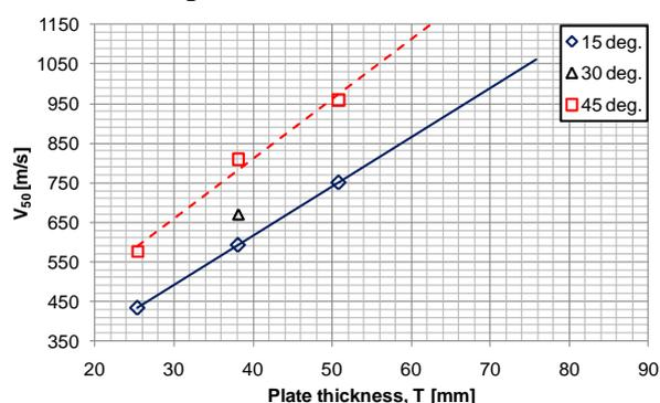
**Figure 2:** Ballistic limit velocities vs. Plate thickness and the obliquity  $\theta$  [23].
