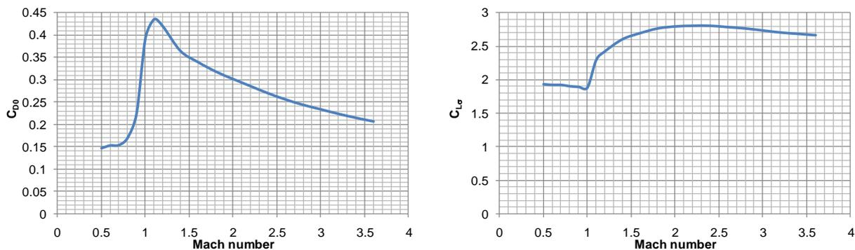
**Figure 9:** Aerodynamic coefficients: axial force (left) and normal force (right).
