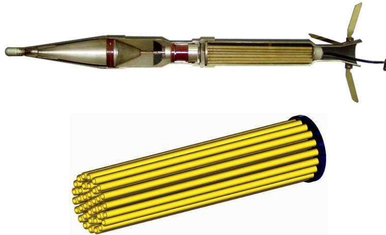
Figure 10. Rocket motor 64 mm M80 (above [19]) and its multiple tube grain (down)
