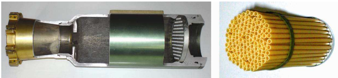
Figure 12. Rocket motor 90 mm M79 (left) and its propellant grain, hollow cylindrical type (right)
