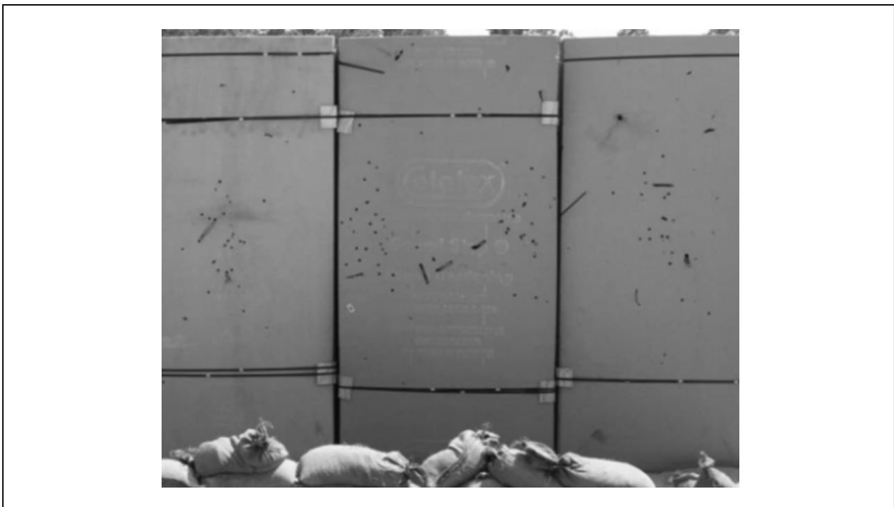
Fig. 21. Effects of natural and embossed fragmentation on Celotex panels after detonation of HE warhead 122 mm 9M22U
