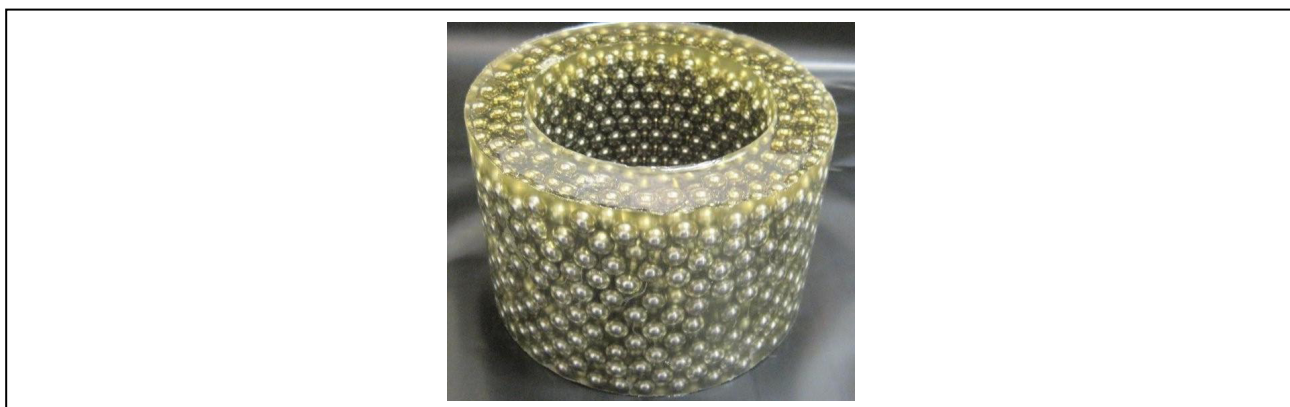
Fig. 14. Preformed fragments (the type of metal) in the matrix cured polymer (Widener et al., 2012).
