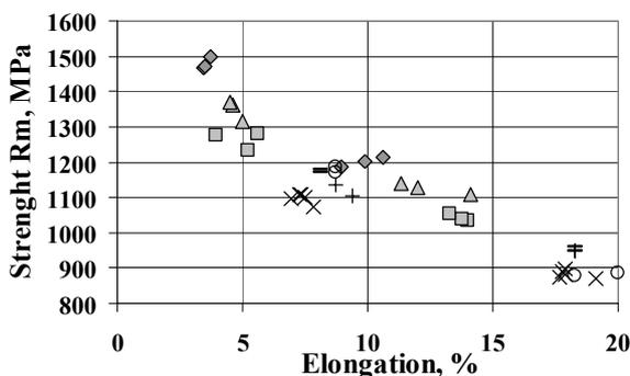
Fig. 3 Tensile strength versus elongation for steels SAE 4130 (full points) and W. No 1.1157
