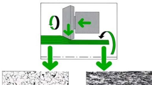
Fig. 1 Crystal grain structure before and after flow forming
