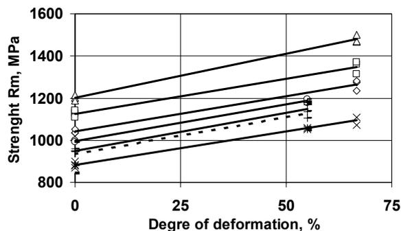
Fig. 2 Tensile strength versus degree of deformation for steels SAE 4130 and W. No 1.1157 (punctual line)
