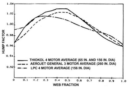
Fig. 2. HUMP factor as a function of the relative web for different rocket motors<sup>[10]</sup>
