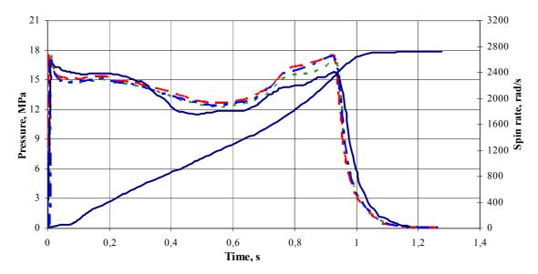
**Fig. 15.** Influence of variation of solid propellant processing on the curve pressuretime form for DB propellant NGR-A tested at temperature of 323 K <sup>[13]</sup>
