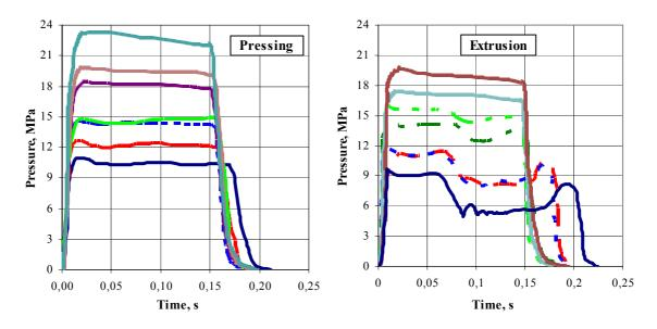
**Fig. 12.** Standardized ballistic evaluation motor 32/16 at temperature of 323 K, propellant NGR-A manufactured by pressing and manufactured by extrusion <sup>[13]</sup>
