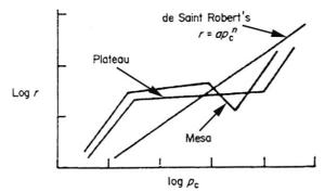
**Fig. 1.** Dependence of burning rate as a function of combustion chamber pressure<sup>[5,6]</sup>
