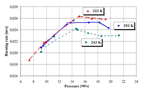
Fig. 13. Kinetic characteristics of the propellant NGR-A (manufactured by continuous process )
