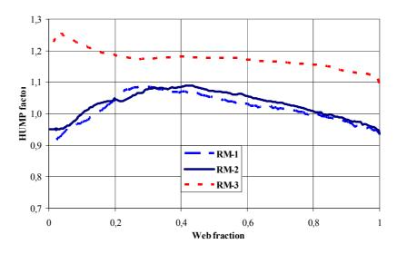
**Fig. 8.** Variation of the basic burning rate under influence of HUMP effect as a function of web thickness for rocket motors 57 mm, *RM-1* and *RM-2* (with central and multiple peripheral nozzles)
