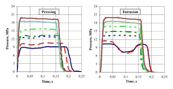
**Fig. 10.** Standardized ballistic evaluation motor 32/16 at temperature of 293 K, propellant NGR-A manufactured by pressing and manufactured by extrusion <sup>[13]</sup>
