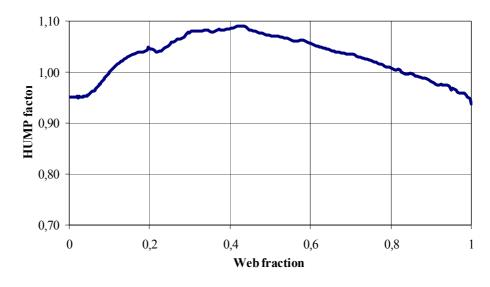
Fig. 6. Influence of the HUMP effect for the rocket motor  $RM-2^{[12]}$
