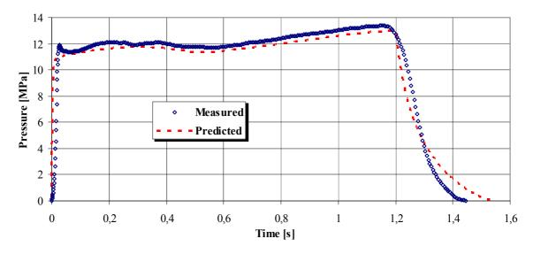
Fig. 7. Pressure-time curve for the motor RM-2, after correction due to HUMP effect <sup>[12]</sup>
