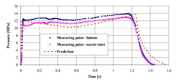
Fig. 5. Pressure-time curve for the test rocket motor  $RM-2^{[12]}$
