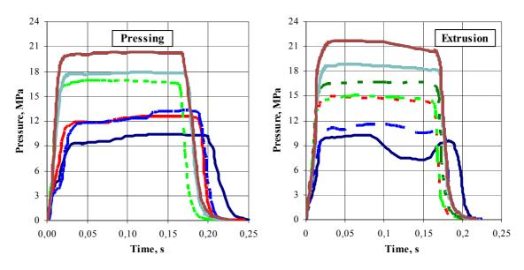
**Fig. 11.** Standardized ballistic evaluation motor 32/16 at temperature of 243 K, propellant NGR-A manufactured by pressing and manufactured by extrusion <sup>[13]</sup>
