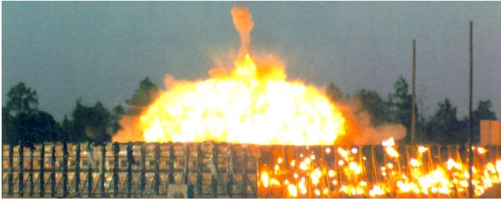
**Fig 4.** Arena fragmentation test (measurement the fragments concentration density per m<sup>2</sup>)
