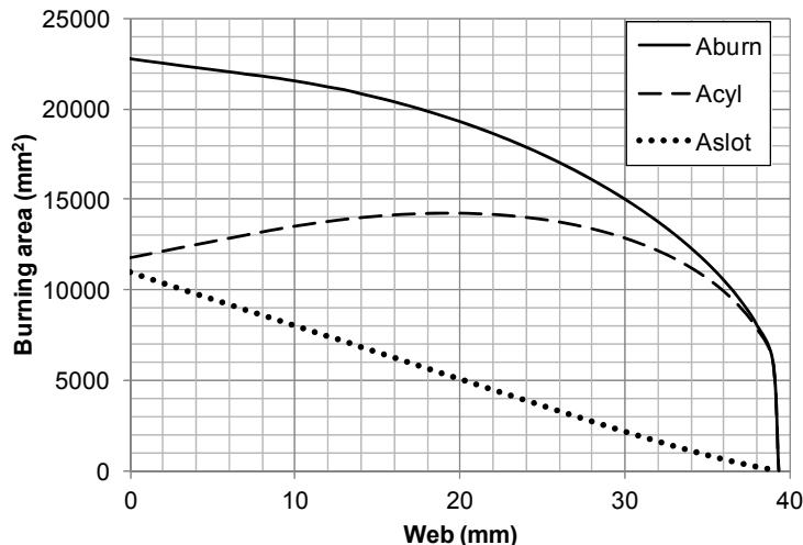
Figure 6: Grain burning surface areas as a function of web
