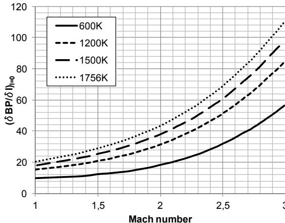
**Figure 2:** Change in base pressure for change in injection parameter vs. Mach number for low injection rates and various temperature
