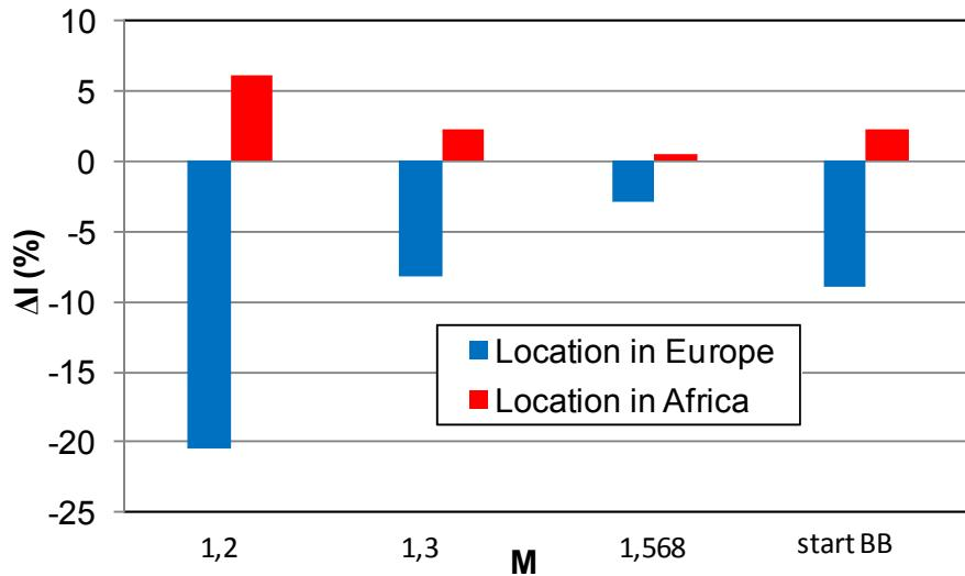
**Figure 9:** Changes of injection parameter for the different locations of launching in percentages
