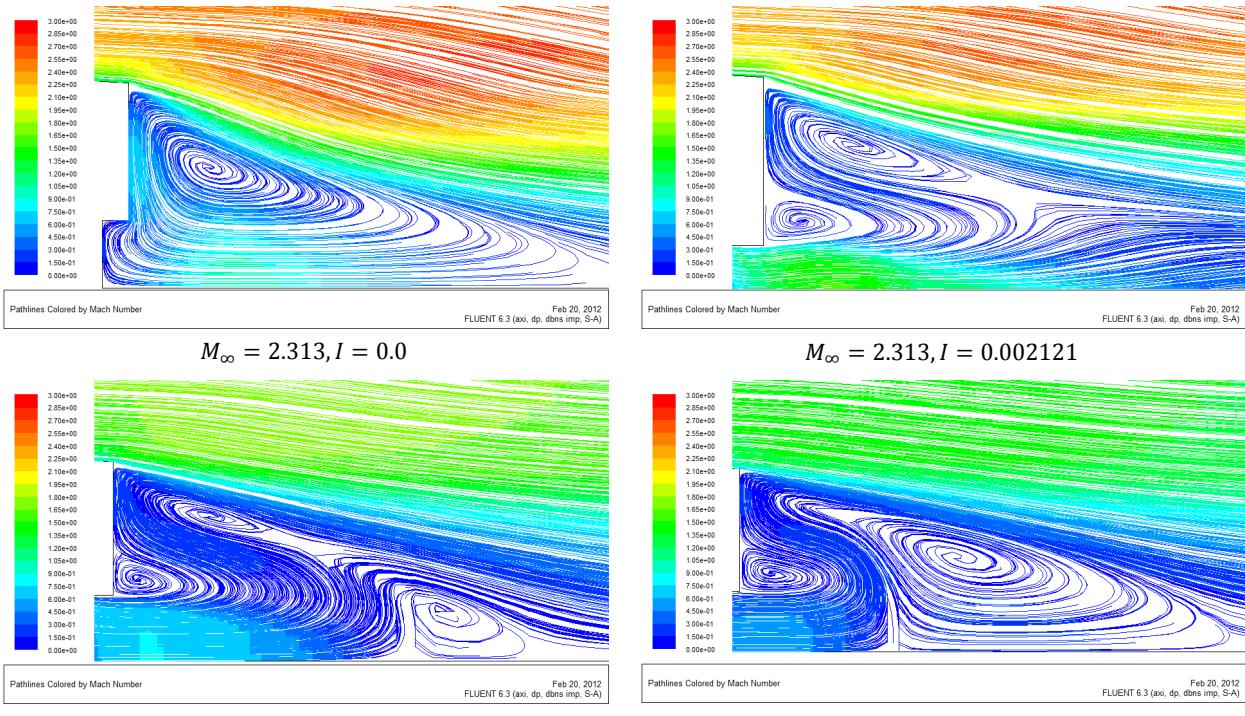
**Figure 8:** Streamlines behind projectile as function of parameter  $I$  and Mach number for the first case
