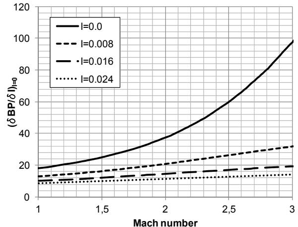
**Figure 3:** Change in base pressure for change in injection parameter vs. Mach number for various injection parameters and  $T = 1500K$
