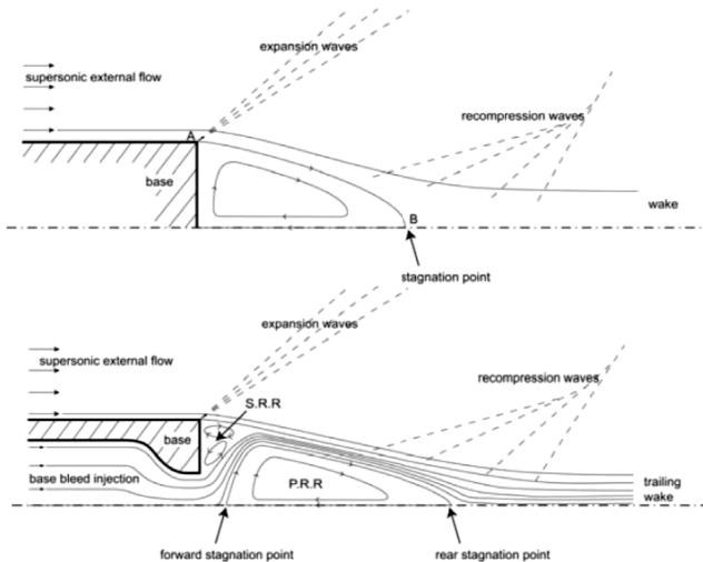
**Figure 1:** Flow field behind a projectile: a) without base bleed; b) with base bleed
