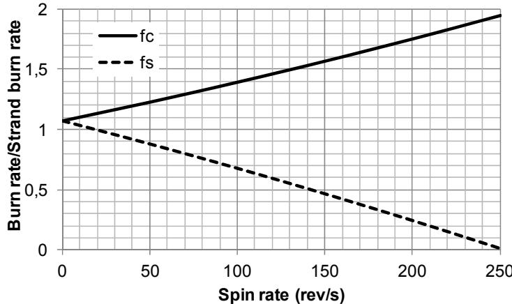
Figure 7: Effect of spin rate on burn rate for the cylindrical and slot surfaces [9]
