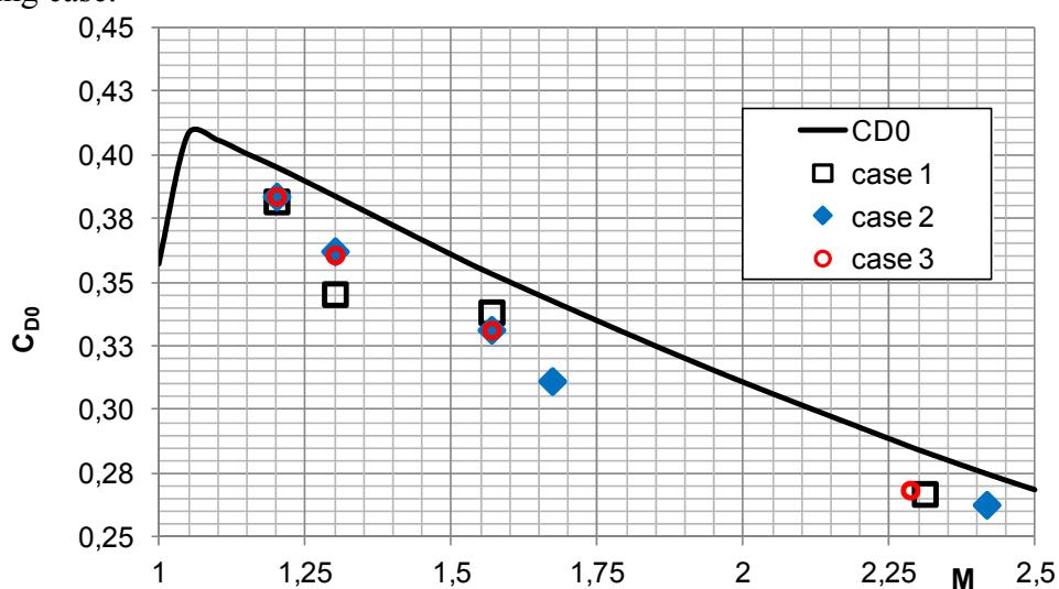
**Figure 10:** Drag coefficient as function of Mach number
