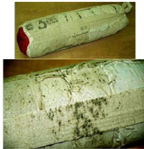
Figure 6. Influence of moisture on bag for propellant charge ammunition 155mm [8]
