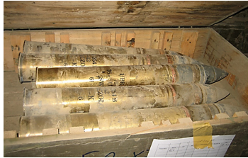
Figure 1. Influence of surface corrosion on AP ammunition 76 mm 345B
