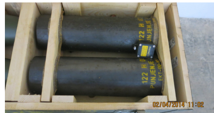
Figure 14. Wooden box with ammunition without internal packing (Eastern concept)
