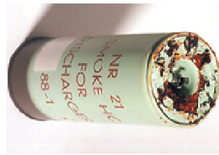
Figure 2. Corrosion caused by moisture on pyrotechnical materials in ammunition [5]
